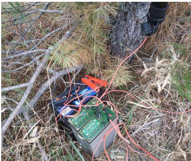
2818. 2021-Sprint: The transmitter of the intermediate beacon, with the spare transmitter and the battery. Top right the bottom of the extensible antenna. The transmitter has the connector for the wire to the antenna and the three radials.
