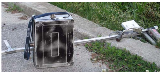
2795. 2006: This equipment operating at 175 MHz was already used in Bulgaria in 2003 and 2006 for reading the SI stations in the field.
